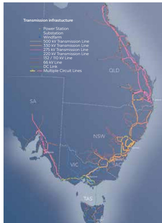
Figure 9: The transmission infrastructure which makes up the National Electricity Market (NEM) in Australia. Image courtesy Australian Energy Market Operator.
