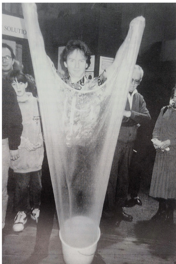
Fig. 5. Rod (R.J.) Binnington demonstrating the extraordinary extensional behaviour of a 2.2% polyacrylamide solution in glycerine/water. Rod was a very gifted experimenter who worked with David Boger at Monash and Melbourne. The photograph was taken at a Science Festival in Melbourne, 1993. (Copyright unknown.).
